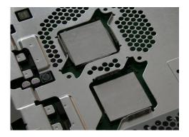
Put <u>one</u> Liquid MetalPad (after the cut) on each processor and then install the cooler on the processor.
