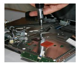
As soon as the four screws of the arrestor of the cooler have to be unfixed, the cooler can be detached carefully. The heat conduction paste, which was applied from the manufacturer, can possibly arrange a strong hold between cooler and processors. Therefore please move the cooler carefully a bit to left and to the right side. After short time and less expenditure of energy you can detach the cooler.
