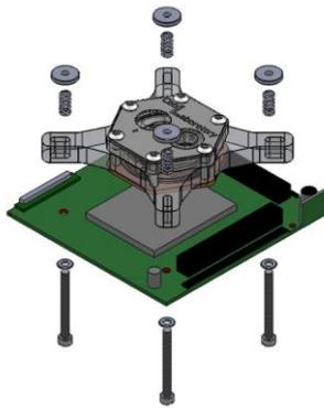
Put heat conduction medium on your processor und insert the screws through the specified assembly drillings. The base surface should rest flat upon on the processor now. Put on the compression springs to the screws and turn the knurled nuts on the screws until they get into contact to the springs. Now turn always the diagonally facing knurled nut to a complete stop and turn each knurled nut a rotation back to be able to realize the maximum contact pressure.
